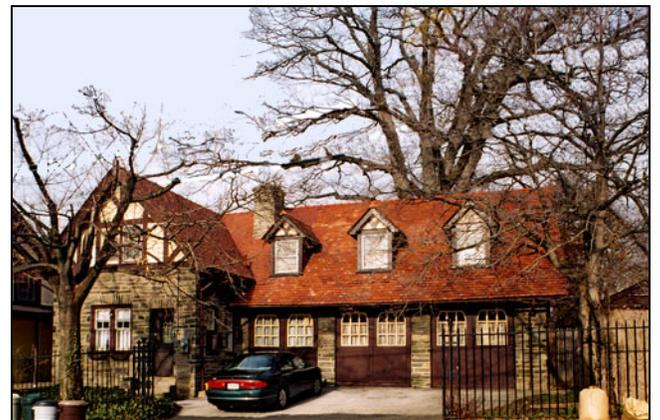
*The terra cotta roof tiles are a distinctive and dramatic feature of this Tudor Revival residence. Also note the overhanging eaves, gable roof dormers and stone chimney protruding at the roof ridge.*
