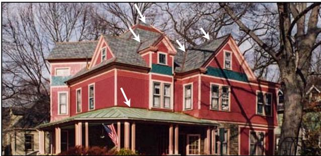
*The arrows indicate typical flashing locations.*
