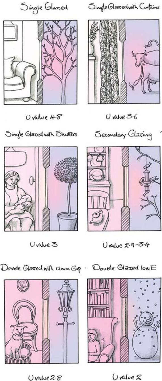
Different U-factors for alternate window configurations and treatments (Note that this graphic originates from the United Kingdom, where the U-Factor is referred to as the U Value. Graphic is from "Energy Conservation in Traditional Buildings," printed by English Heritage in 2008. Accessible at [http://www.climatechangeandyourhome.org.uk/live/content\\_pdfs/526.pdf](http://www.climatechangeandyourhome.org.uk/live/content_pdfs/526.pdf)).
